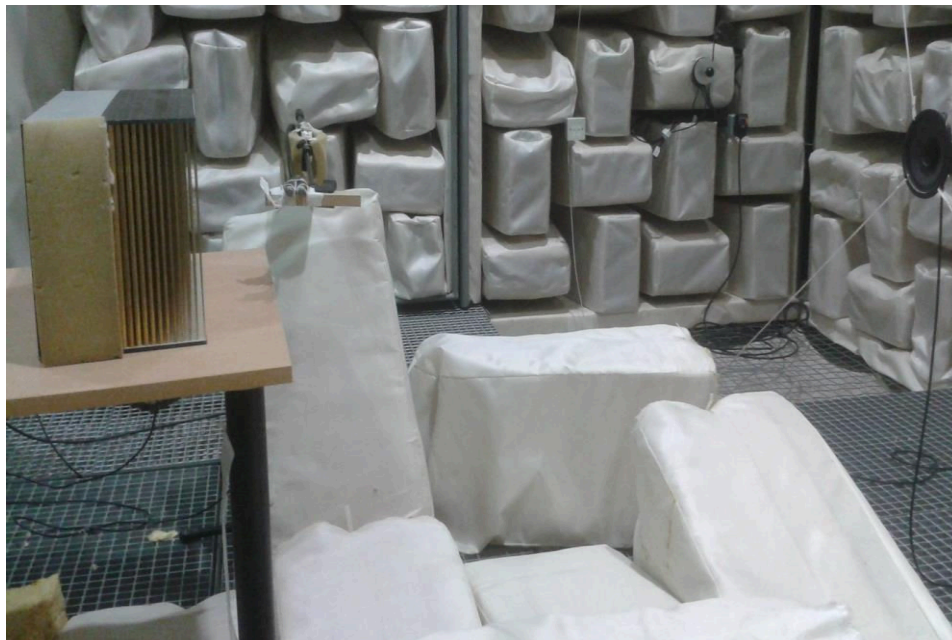
Fig. 3. Photograph of the experimental set up showing the QFAA (left) and the loudspeaker (right).
