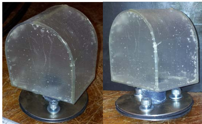
Figure 8 - 3D printed Helmholtz resonators with attachment panels.
