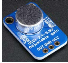
Figure 7 - Commercial electret microphone and built in amplifier
